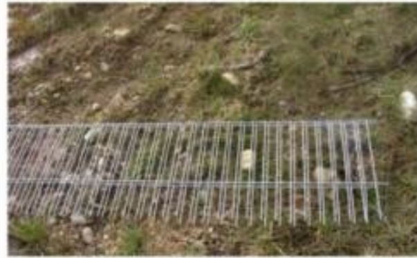
Figure 2.2. Detail of an appropriate electro-welded mesh.
